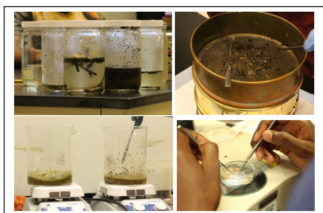
Fig. 2. Density sample processing: collected sample; sieving, Fenton Reaction digestion; microplastic sorting.
