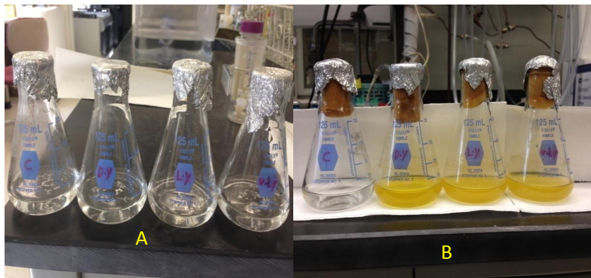
Fig.1 Microcosms to assess Dibenzofuran biodegradation A: day 0, B: day 7, note: Letter ( c) on the flask means control other flasks are three live replicates.
