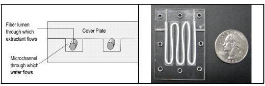
**Figure 1.** (a) Design of the Microfluidic Extractor. (b) Photograph of the device compared to a US quarter.
