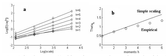
Fig. 5. Scaling of precipitation (a) and the non-linear structure function indicative of a multifractal process.
