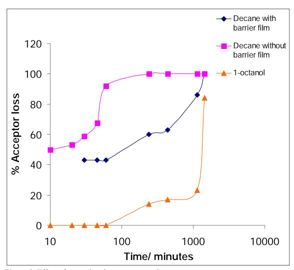
Figure 2. Effect of extraction time on acceptor loss.
