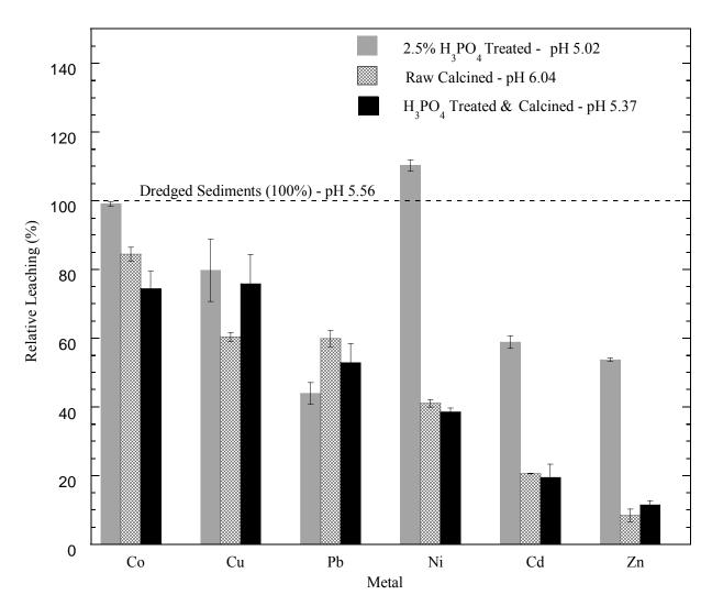
Figure 3. TCLP metal leaching for sediment treatments relative to amount leached from dredged sediments. Percent of leaching from calcined sediments are adjusted for loss of organic matter. Error bars indicate  $2 \times \text{standard error}$ . Lower pH after phosphoric acid treatment increased Ni leaching as compared to dredged sediments.
