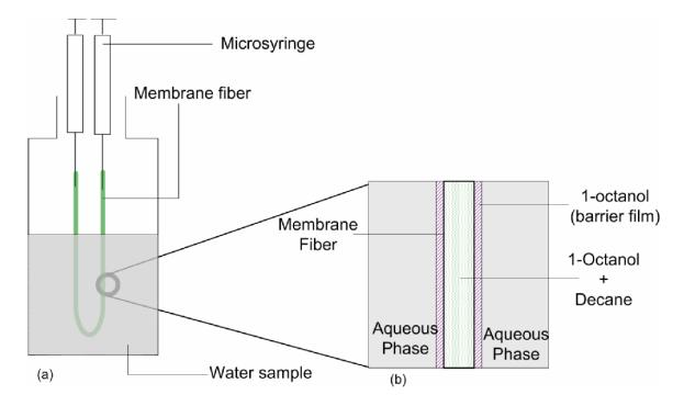
**Figure 1.** (a) Experimental set-up for microextraction of N-methyl carbamates; (b) Schematic diagram of the barrier film system. Membrane lumen contains a mixture of solvents whose loss is reduced by the presence of the 1-octanol film.
