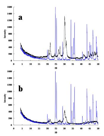
Figure 2. X-ray diffraction patterns collected for Pb minerals before (blue line) and after (black line) the reaction. The X-ray diffraction patterns in blue and black correspond to cerussite (PbCO $_3$ ) and hydroxy-pyromorphite [Pb $_5$ (PO $_4$ ) $_3$ OH], respectively. a) experiment with culture medium and soil bacterium GP-19S; b) control experiment with culture medium alone.
