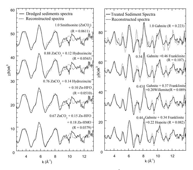
Figure 2. Experimental and LCF reconstructed  $\chi(k) \cdot k^3$  spectra for dredged and treated sediments. Only spectra with more than 10% contributions are included. The fitting factor  $R = \sum [(k^3 \chi_{exp} - k^3 \chi_{model})/k^3 \chi_{exp}]^2$  where  $\chi_{model}$  refers to spectra reconstruction with PCA decomposed components.
