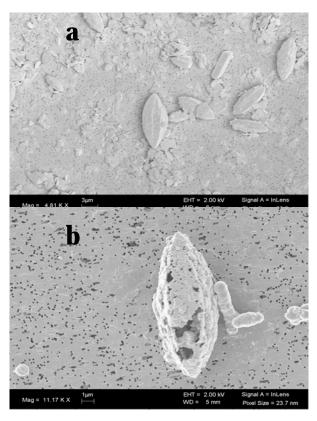
Figure 1. SEM images of cerussite (PbCO<sub>3</sub>) before and after reaction in a culture medium with the soil bacterium GP-19S. a) cerussite particle at the beginning of the experiment; b) cerussite particle at the end of a two week incubation.
