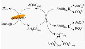
(c) Abiotic arsenate reduction coupled to iron oxidation can result in the capture of arsenate, arsenite, and phosphate. Arsenite binds to ferric iron, but more weakly than arsenate.
