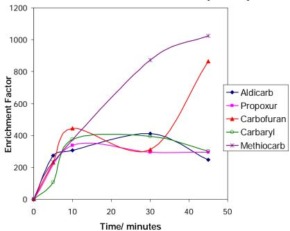
**Figure 4.** Effect of extraction time on enrichment factor. Sample spiked with 10ppb of pesticides and 40/60 1-octanol/decane (v/v) used as organic acceptor. Stirring speed is 80rpm.
