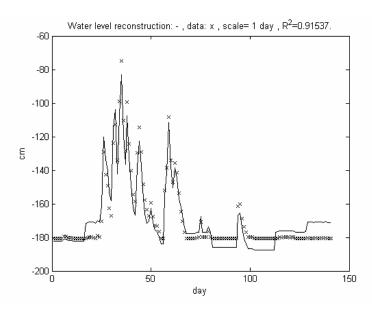
**Fig. 6**. Groundwater level fluctuation reconstructed with an inverse wavelet transform using precipitation data to predict the base function of groundwater at decomposition level 6 (see Fig. 3 and Table 3).
