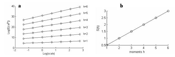
**Fig. 4**. Scaling of groundwater level (a) and the linear structure function indicative of a fractal process (b).
