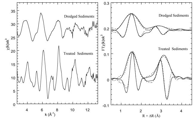
Figure 1. Dredged and treated sediments: (a) Background subtracted, normalized, and averaged  $\chi(k) \cdot k^3$  spectra and (b) Fourier transformation  $\chi(k) \cdot k^3$  (solid lines) over 3.0–12.5 Å<sup>-1</sup> and fitted (dashed lines) with models.
