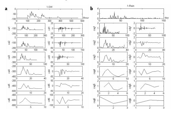
**Fig. 3**. Decomposition with wavelet Haar of a) groundwater level and b) rainfall of site 1. Symbols in the y-axis:, 'ca' and 'cd' refer to the low frequency signal (base, B(t)) and the high frequency signal (noise, A(t)), and l and g stand for rainfall and groundwater, respectively. The numbers represent the levels or number of applying wavelet transformation.
