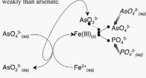
(d) Spontaneous formation of ferrous arsenates (e.g. symplesite) and ferrous phosphates (e.g. vivianite) is likely to occur, resulting in capture of arsenate and phosphate.
