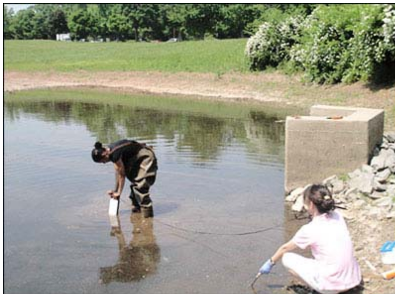
Bernice Rosenzweig deploying a porewater sampler near the outlet of the Princeton University Campus Detention Pond. Visiting researcher, Hee Sun Moon looks on.
