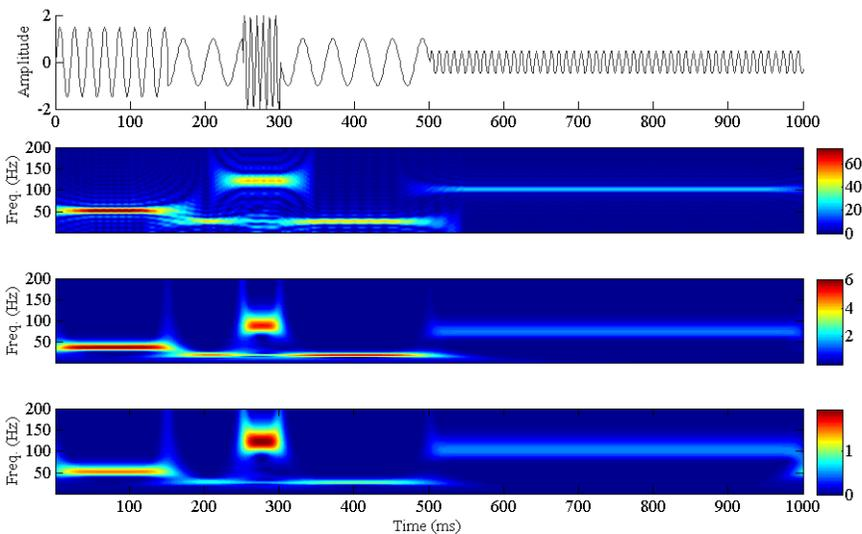
Time – Frequency analysis for a synthetic signal (a) time series, (b) STFT section, (c) WT section and (d) ST section.
